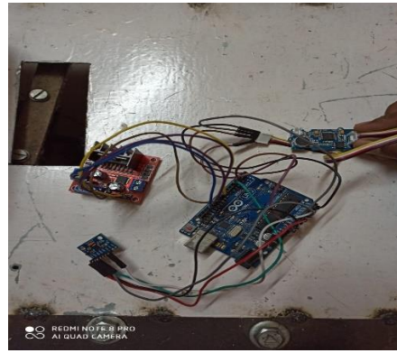
The connection of MPU6050, L298N and Motor Drive to Arduino Uno3
