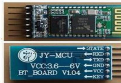
Figure. 3: Bluetooth Module (HC-05) [3]
