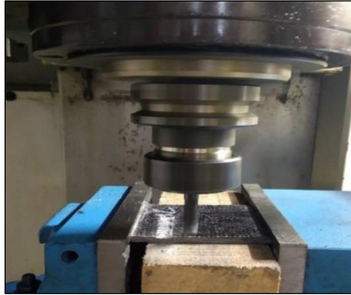
Fig. 1. Machining (Milling) for MWCNT doped epoxy and Glass fiber in polymer composites
