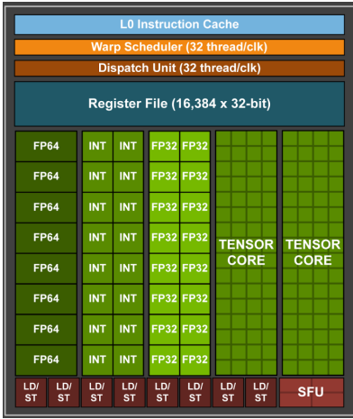
Fig. 2. A processing group of the Nvidia Tesla V100 which has a total of 640 tensor cores. Image taken from the Nvidia CUDA programming guide [16]
