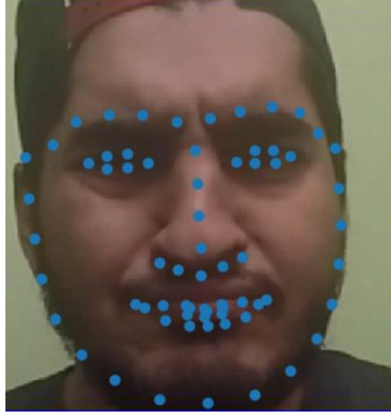
Figure 6: 68 fiducial points superimposed on the detected face
