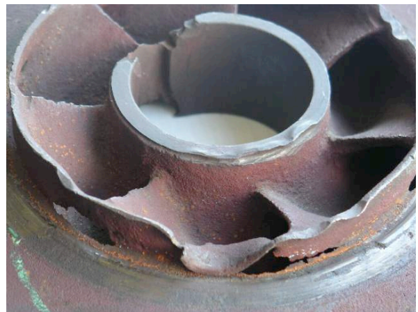
Figure 4: Centrifugal pump destroyed by cavitation
