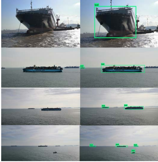
Fig. 4. Bounding box with a green rectangle is the notation used during SSD training.
