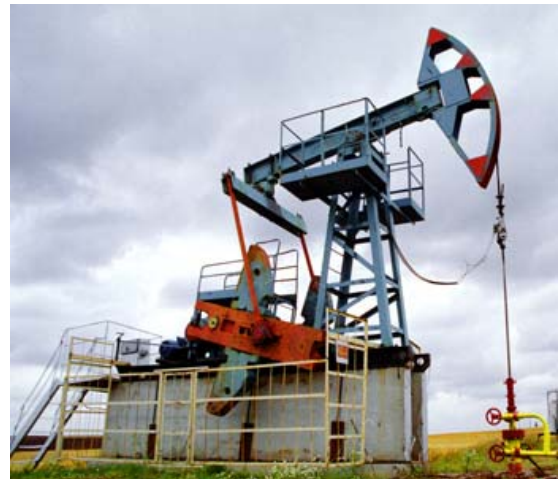
Fig.1. Sucker-rod pump unit
