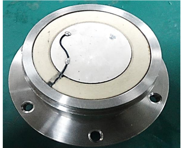
Figure 4 Echo sounder prototype before molding
