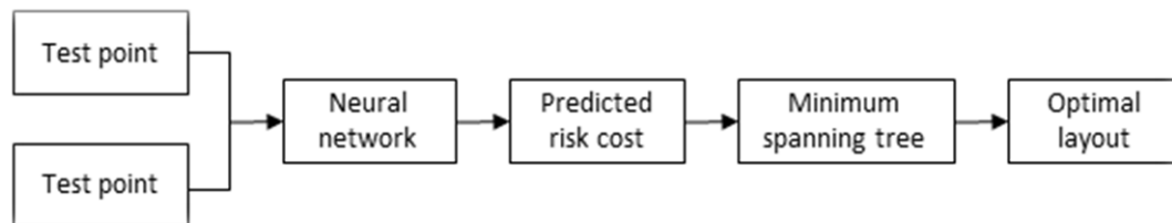
Figure 5. Procedure for solving for the optimal layout of a pipe network
