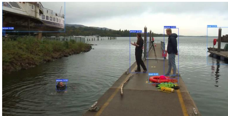
Fig. 2. Object detection by YOLOv7 when human partially submerged on water.
