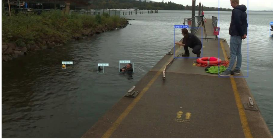
Fig. 3. Misclassified partially submerged human.
