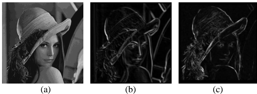
Fig.5. Image decomposition. (a) Input image. (b) Decomposition image with stepped edge elementary manifold. (c) Decomposition image with Gabor basis function manifold.
