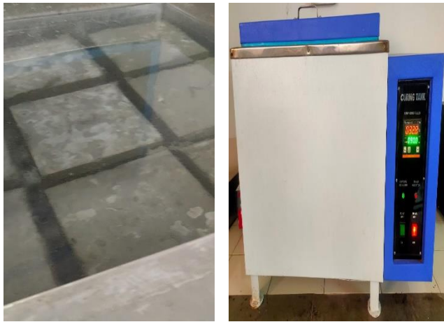
Fig.2. Specimen Cubes Subjected to Curing at 90 °C in hot water machine.
